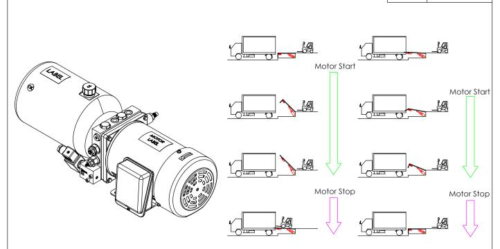
"Dock Leveller" Hydraulic Valves Diagram
